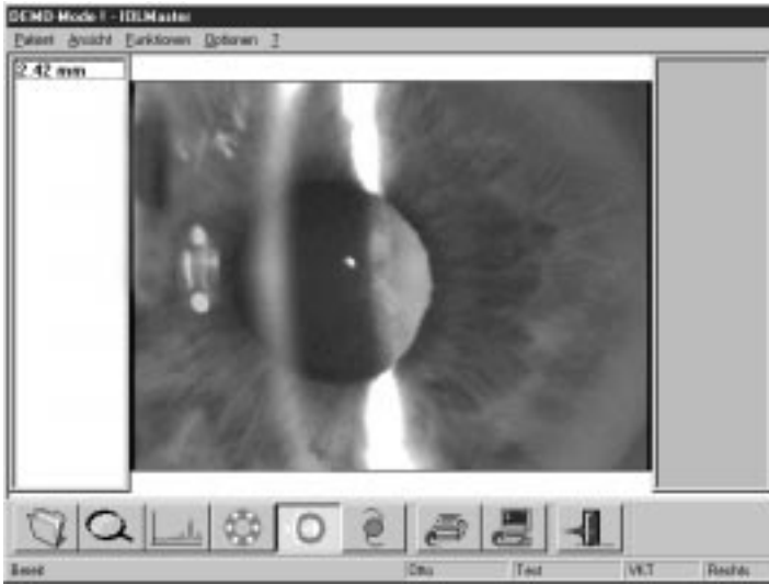
Figure 5 Screen display of the IOLMaster in anterior chamber depth measurement
